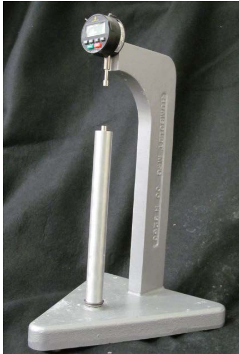
Fig. 3. Spacer rod used to accommodate smaller specimens using the same stand as for C1012.
