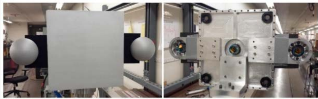
Fig. 5. Fourth prototype of the plate-sphere artifact with two 100 mm diameter integration spheres mounted on the sides of a square plate with side dimensions of 304.8 mm (12 in.).
