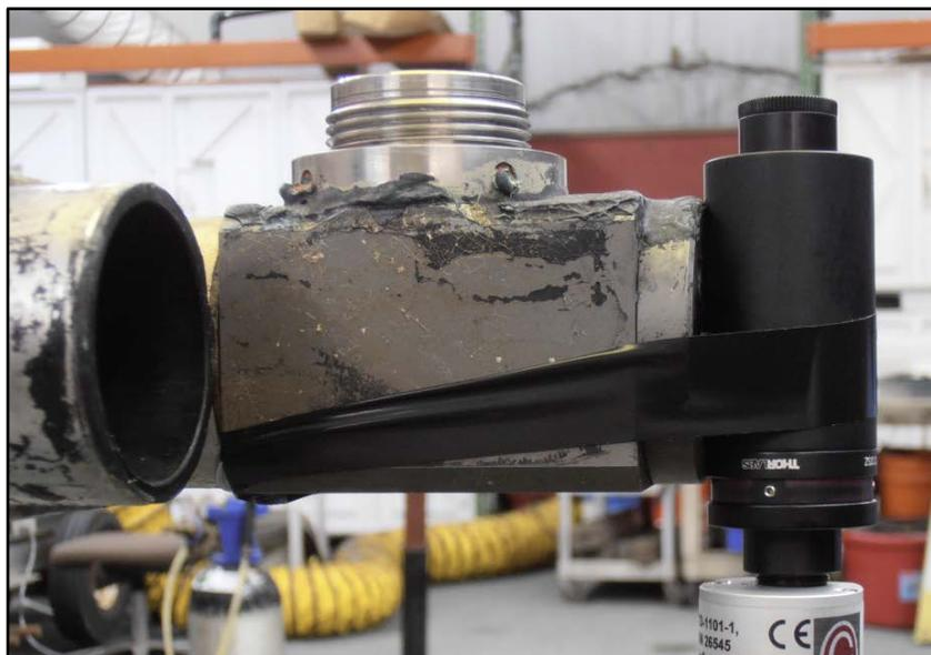
**Fig. 2.** Photograph of the MOBY radiance collector, which was used without the antifouling tube, during the setup of the immersion experiment. The shell of the buoy arm is to the left, and the monitor photodiode is to the right.
