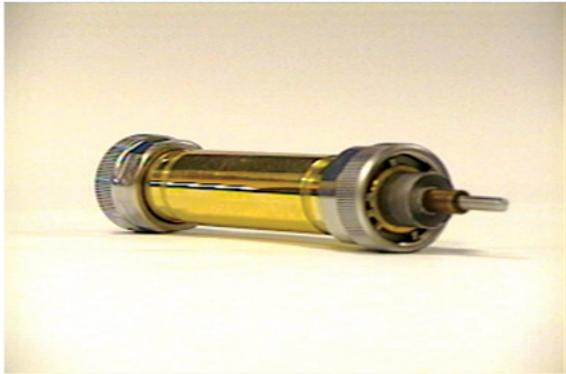
Fig. 23. A typical coaxial line with a specimen inserted.
