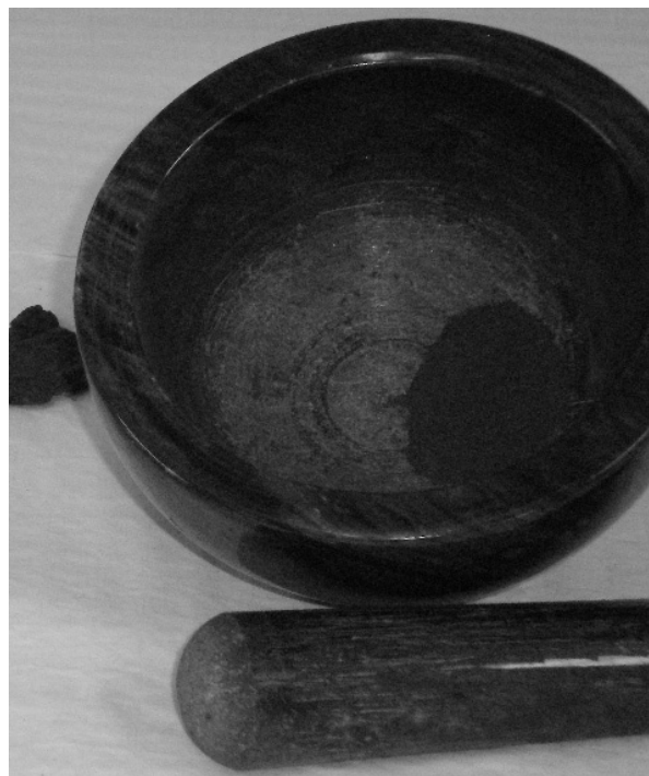
Fig. 9. Corrosion powder ground from samples taken from girders.
