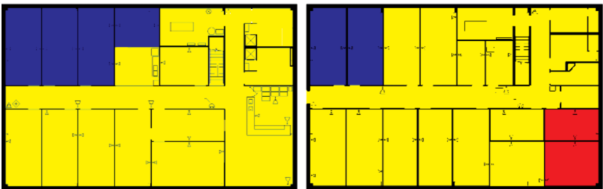
Fig. 23. Cluster 4 Zoning strategy of 1st and 2nd Floor for scenarios with 2nd Floor Office Release and Supply Fans ON (Red = Class 1, Yellow = Class 2, Blue = Class 3).
