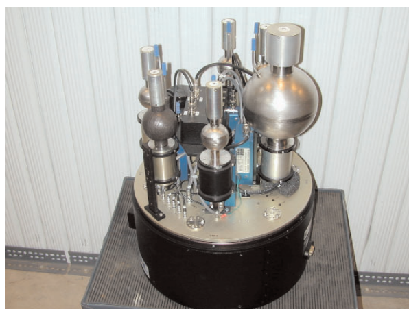
Fig. 1. Base ROSPEC with six proportional counters.
