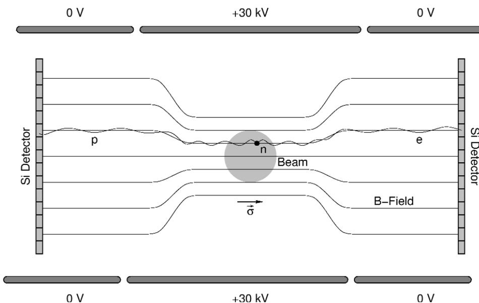
Fig. 2. The conceptual design for the spectrometer showing the most important elements (not to scale). The beam direction is into the page.
