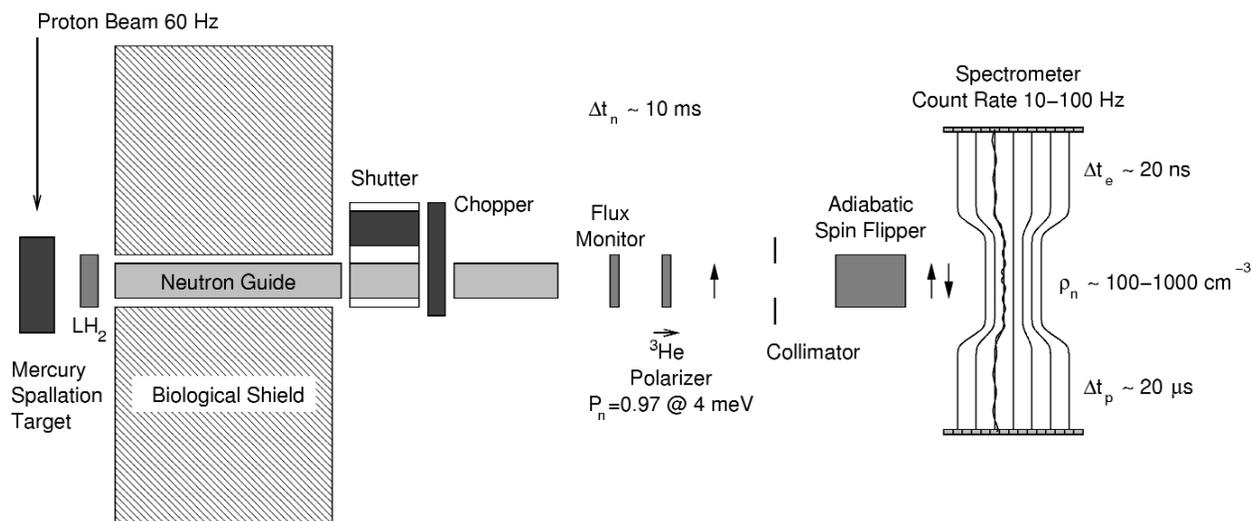
Fig. 1. The conceptual design for the abBA experiment, shown in the SNS (polarized neutron beam) configuration.
