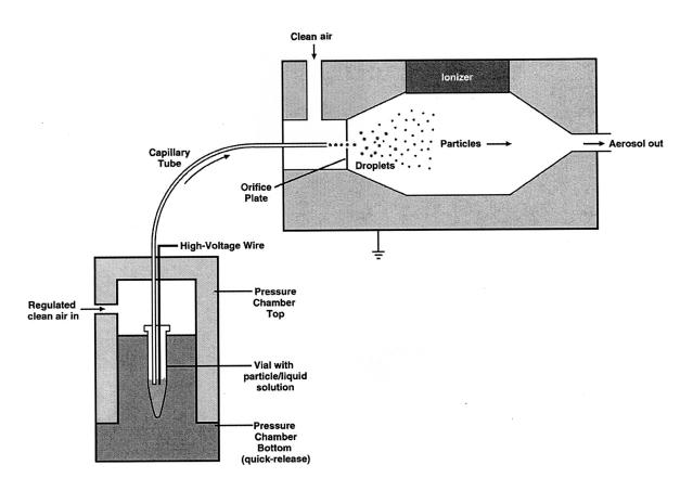
Fig. 1. Schematic diagram of the electrospray adapted from the TSI 3480 technical manual.
