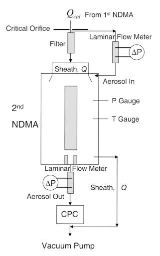
**Fig. 3.** Schematic diagram of the measurement NDMA system for reduced pressure conditions.
