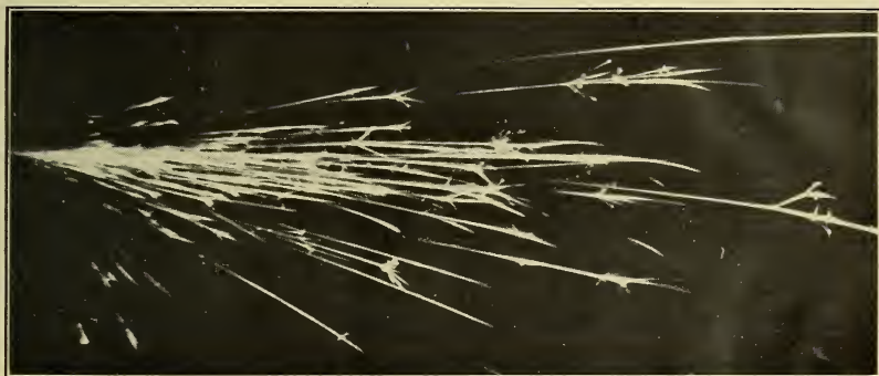
FIGURE 14.— Spark stream typical of chromium-nickel steel. Type S.A.E. 3130, c.f. (fig. 4).
