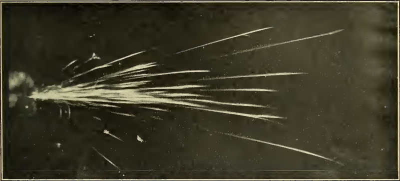
FIGURE 2.— Spark stream of open-hearth iron. Enlargement of 1A.
