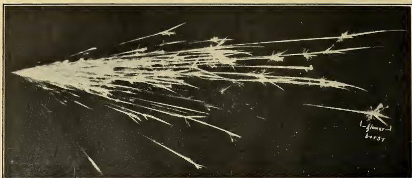
FIGURE 10.—Spark stream of typical chromium steel showing the flower burst. Type S.A.E. 5140, c.f. (fig. 4).
