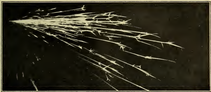
FIGURE 19.— Spark stream typical of chromium-vanadium steel. Type S.A.E. 6130 steel, c.f. (fig. 4).
