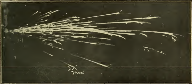
FIGURE 25.—Spark stream typical of silico-manganese steel, showing jacketing effect. Type S.A.E. 9250.
