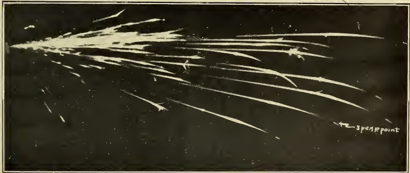
FIGURE 21.— Spark stream typical of molybdenum steel, showing spearpoints. Type S.A.E. 4130, c.f. (fig. 4).
