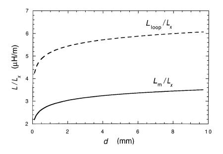
**Fig. 4.** A comparison of the magnetic inductances per length for a conducting sheet and return wire,  $L_{\rm m}/L_x$ , and for a conducting wire and return wire,  $L_{\rm loop}/L_x$ , when using separation distances *d* between 0.1 mm and 10 mm, the parameters listed in Sec. 2.2 for  $I_{\rm SD} = 25 \ \mu$ A, and assuming that the wire radius  $\rho$  is 2.5 nm.
