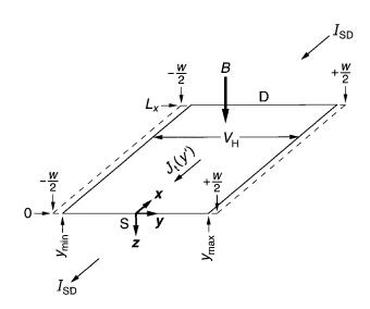
**Fig. 1.** A 2DEG conducting sheet, with the origin of the coordinate system located at the source S, halfway across the device width w. The device length is  $L_x$ , and D is the drain. Conducting electrons extend across the device from  $y_{min}$  to  $y_{max}$ . *B* is the external magnetic flux density,  $V_{\rm H}$  the quantum Hall voltage,  $I_{\rm SD}$  the applied current, and  $J_t(y')$  the total current density at point x', y', 0 in the 2DEG.
