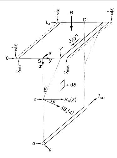
**Fig. 3.** A sketch of the 2DEG conducting sheet and a parallel current return wire of radius  $\rho$ , located a distance *d* from the middle of the sheet.  $B_s(z)$  and  $B_w(z)$  are magnetic flux densities generated by the conducting sheet and wire. dS = dxdz is an elemental area in the x-z plane located between the conducting sheet and the wire.
