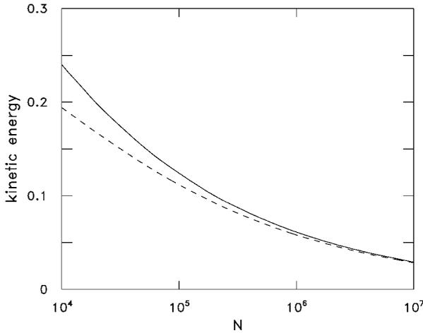
**Fig. 5.** Kinetic energy per particle, in units  $\hbar\omega_{\text{HO}}$ , for  $^{87}\text{Rb}$  in a spherical harmonic trap as a function of the number of condensed atoms. Solid line: from the solution of the Gross-Pitaevskii equation (1). Dashed line: approximation Eq. (16).
