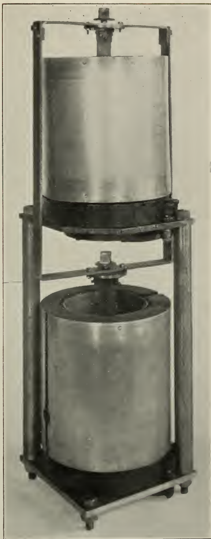
FIGURE 9.—Apparatus for the determination of the temperature coefficient of Young's modulus of elasticity
