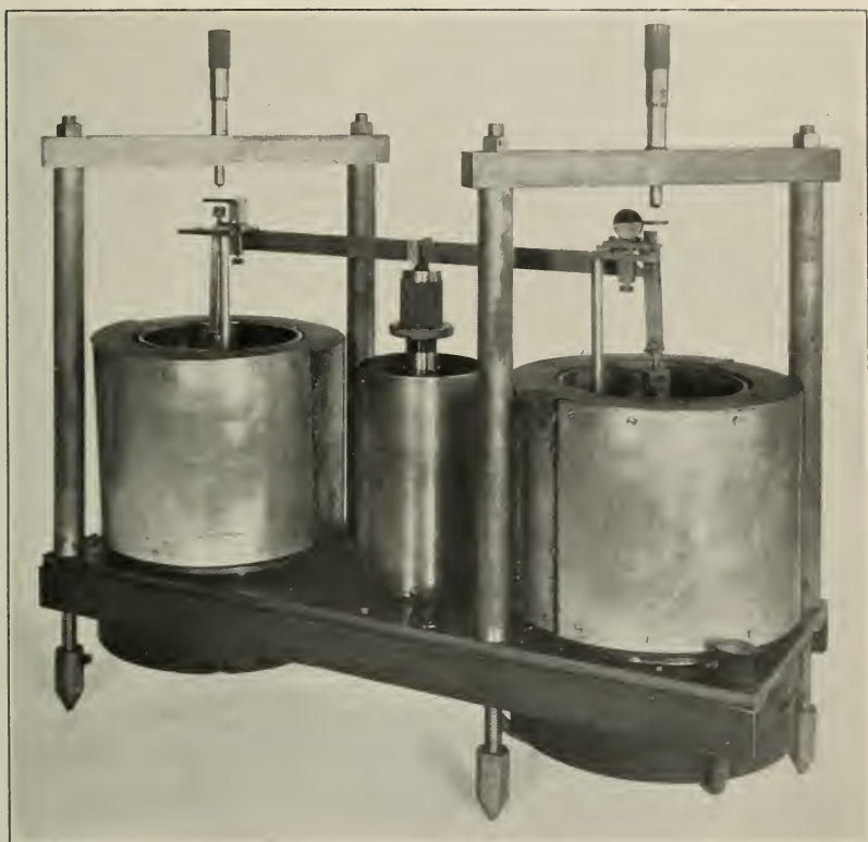
FIGURE 3.— Apparatus for the determination of the temperature coefficient of the rigidity modulus
