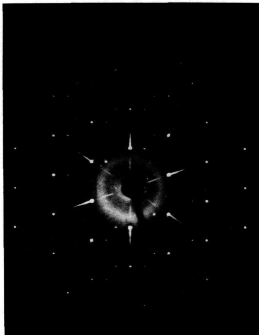
Fig. 7. X-ray precession photograph of the fcc  $\alpha_1''$  phase (Mo radiation).
