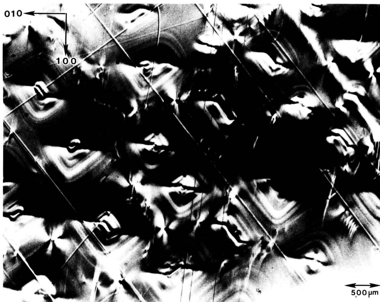
Figure 14. Magnified portion of image of diffraction in Laue geometry at 10 keV from (400) planes of the (001)-cut indium doped gallium arsenide crystal shown in figures 2, 3, and 13.
