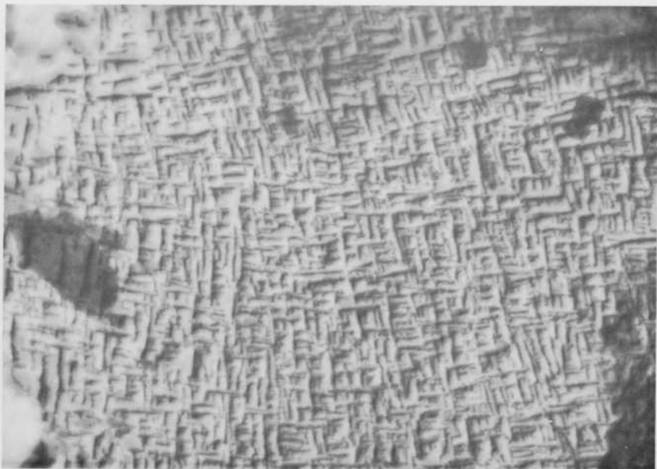
FIGURE 21. Magnified view of central portion of replica shown in figure 20. Note dense but not compact network of intercrossing structural units. \times 39000 .
