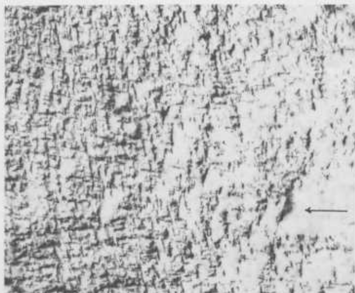
FIGURE 38. A view at higher magnification of a portion (note arrow) of the replica shown in figure 37, revealing the cross-hatched surface texture of the replicated aggregate. ×33200.
