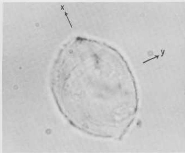
FIGURE 8. Crystalline aggregate grown from a 0.75 percent solution of polypropylene in mineral oil at 112 °C. Note elliptical profile of aggregate when seen as depicted here along an axis (z) at right angles to its plane (x,y) of preferential development. Unpolarized light, \times 1,930 .
