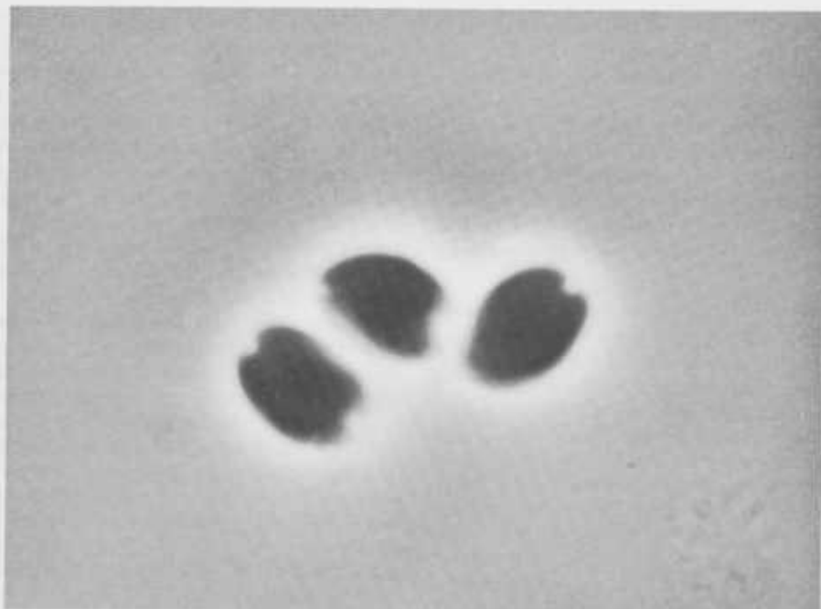
FIGURE 36. Notched aggregates grown from a 0.01 percent solution of polypropylene in amyl acetate at 100 °C. Phase Contrast \times 2100 .
