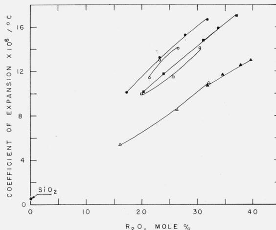
FIGURE 7. Average coefficient of expansion of binary alkali silicate glasses and fused silica for the temperature interval  $50^\circ$  to  $400^\circ C$ .
