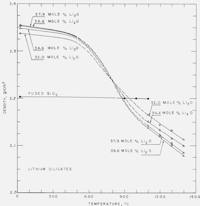
FIGURE 2. Densities of binary lithium silicate glasses and liquids and fused silica as a function of temperature.
