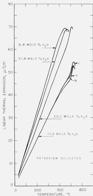
FIGURE 5. Linear thermal expansion of binary potassium silicate glasses.
