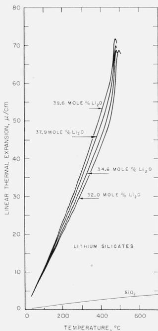
FIGURE 1. Linear thermal expansion of binary lithium silicate glasses and fused silica.
