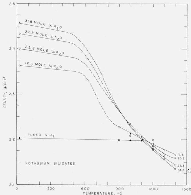
FIGURE 6. Densities of binary potassium silicate glasses and liquids and fused silica as a function of temperature.
