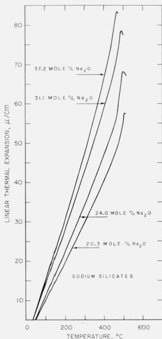
FIGURE 3. Linear thermal expansion of binary sodium silicate glasses.
