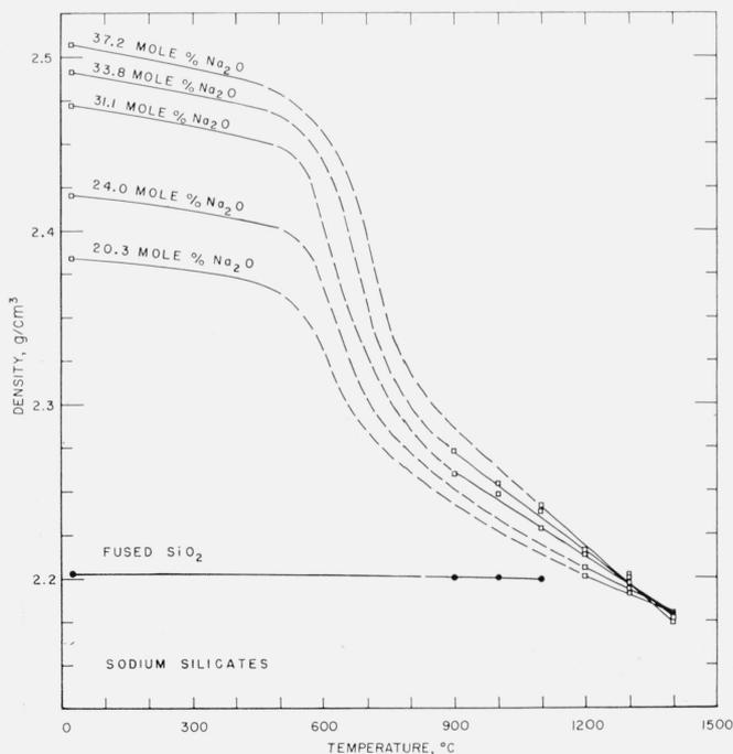
FIGURE 4. Densities of binary sodium silicate glasses and liquids and fused silica as a function of temperature.
