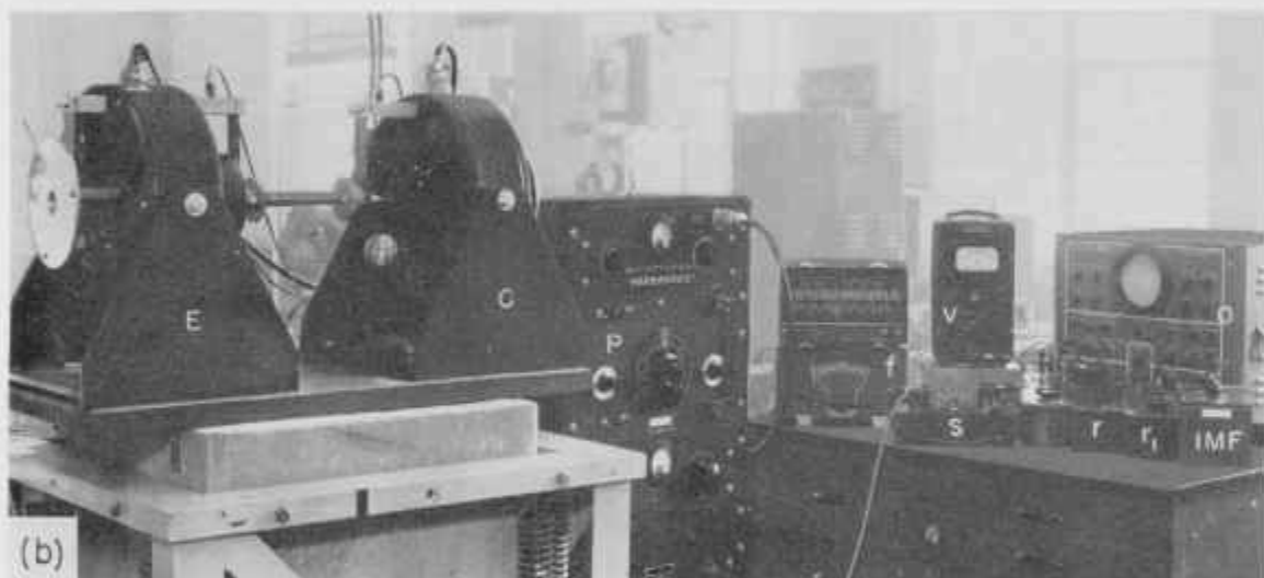
FIGURE 1. Measurement of constants of vibration-pickup calibrator.
