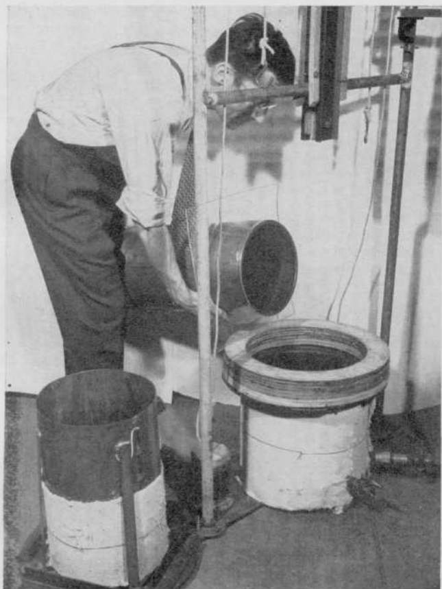
FIGURE 3. Vacuum-forming apparatus partly disassembled after forming a sheet of acrylic plastic.
