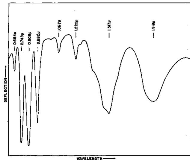
FIGURE 1. The absorption spectrum of didymium glass under prism dispersion from 0.6 to 2.0  $\mu$ ;  $t=0.6$  mm.
