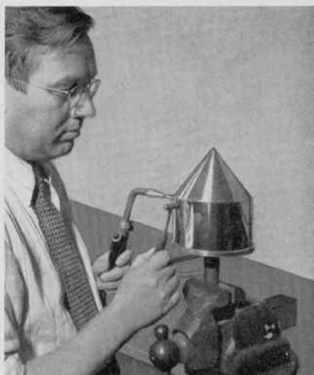
FIGURE 3. Cylindrical crucible with conical base. Platinum walls being welded together on a steel mandrel.
