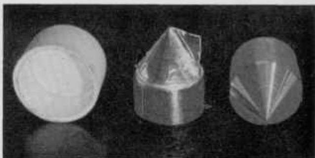
FIGURE 7. Platinum crucible (center) showing radiation fin welded to cone portion of crucible.
