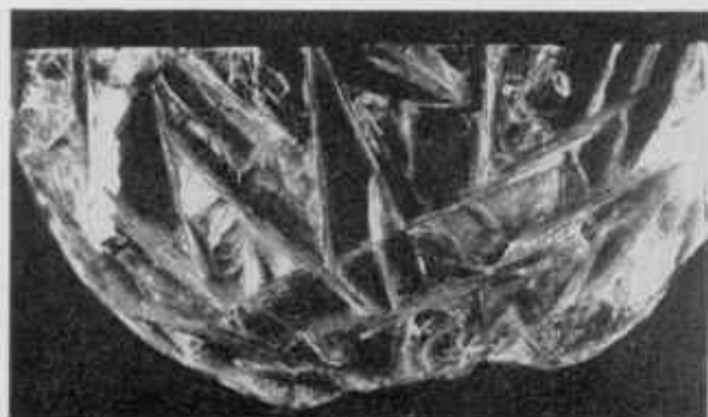
FIGURE 9. A view of the horizontal surface (one-half cake) of a large mica melt, showing good vertical orientation but lack of parallel orientation.
