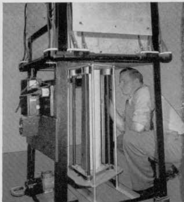
FIGURE 5. Large Glocar Crystallizing furnace with elevator lifting apparatus underneath.
