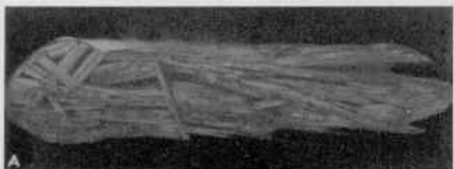
FIGURE 9. A view of the horizontal surface (one-half cake) of a large mica melt, showing good vertical orientation but lack of parallel orientation.
