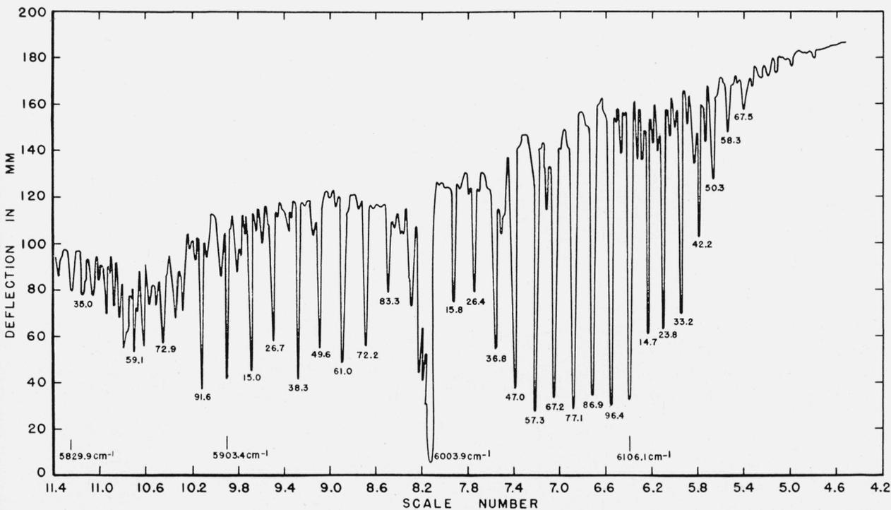
FIGURE 2. Absorption spectrum of the 1.66- $\mu$  band  $\text{CH}_4$ .
