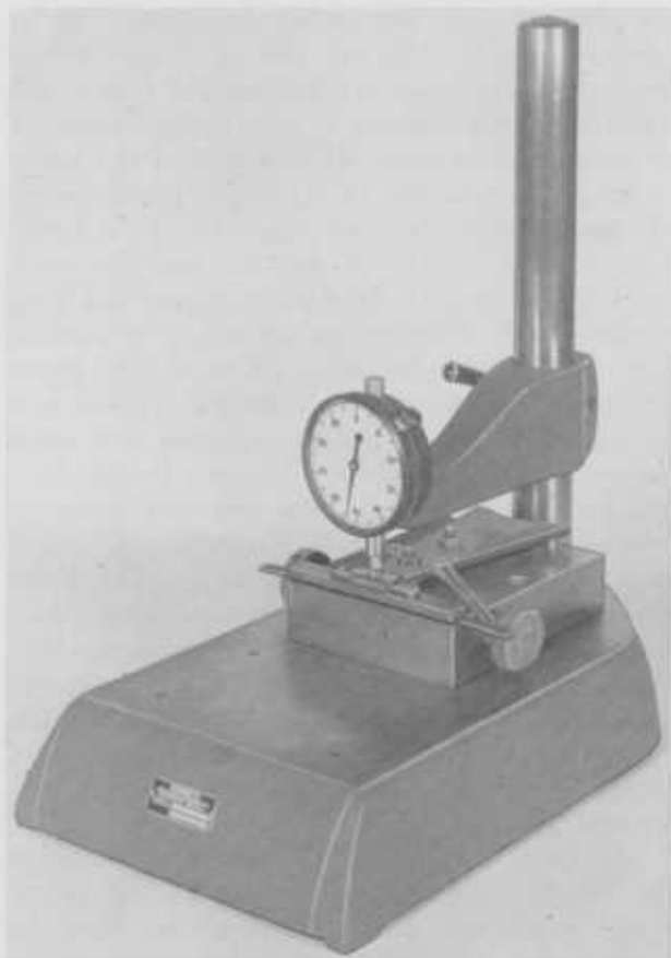
FIGURE 3. Gauge for obtaining average thickness of the specimen.
