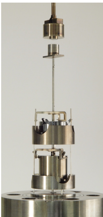
Fig. 3-4. Sinkers in the two-sinker densimeter (shown removed from the measuring cell). The titanium sinker is on the bottom, with the tantalum sinker above. The magnetic suspension coupling is at the top of the image; this comprises the electromagnet, which hangs from the balance; and the permanent magnet, which picks up the sinkers via “lifting forks;” the top of the measuring cell passes between the electromagnet and permanent magnet. In this photo, the titanium sinker is suspended off of its rest and is being weighed.
