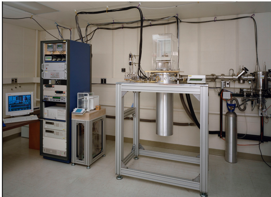
Fig. 3-3. Two-sinker densimeter. The main part of the instrument is to the right of center with the vacuum thermostat below and balance above; the electronics are on the left side; a vacuum system for both evacuating the measuring cell and maintaining the vacuum thermostat is on the right. A separate system for calibrating sinker volumes sits to the right of the instrument rack.
