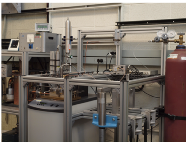
Fig. 3-8. Dual-path, pulse-echo, speed of sound instrument. Shown are the thermostat (left of center, which contains the measuring cell) and the fluid manifold and pressure transducer; a vacuum system for evacuating the measuring cell is to the left of the thermostat.
