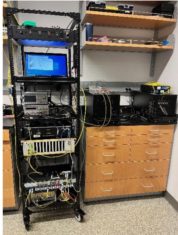
**Figure 110.** Deployed, rack-mounted quantum network node at the University of Maryland. (Photo by T. Gerrits, NIST)
