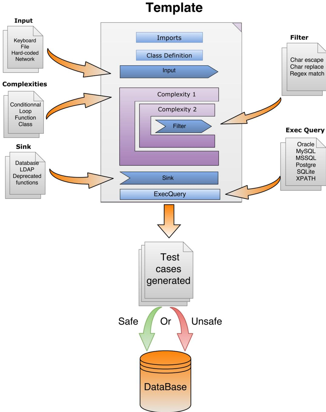
**Fig. 2.** Overview of VTSG test case generation. The File Template specifies how pieces are assembled. Input, Filter, Complexity, Sink, and Execute Query modules provide code. The filter is wrapped with two complexities. An example test case is in Figs. 14 and 15.
