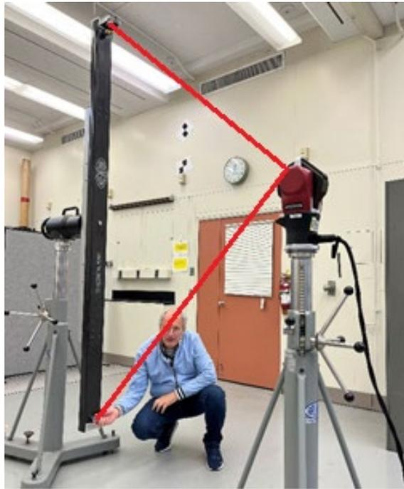
**Fig. 5.** Three-nest scale bar in the vertical position.
