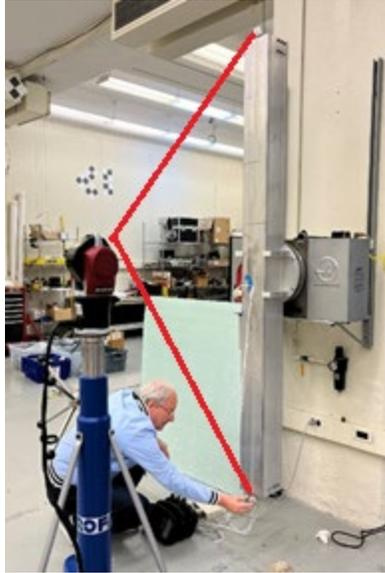
**Fig. 10.** Two-nest scale bar in the vertical position.
