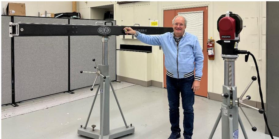
Fig. 4. Three-nest scale bar in the horizontal position.
