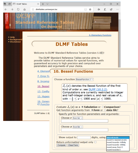
Figure 88. DLMF Tables generates tables of special function values at user specified precision. Users input real values and parameters where the function is to be evaluated. The user may request output in interval mode, where the output is shown as a table of intervals that bound the true results or may request output in one of several rounding modes. Users may also choose to compare their own table of values to the reference values generated by the system.
