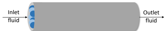
Figure 20. Illustration of break-through curve measurement. A column (grey) is packed with solid particles (blue). Mechanical forces on each end are used to ensure that the solid does not move. After flowing a non-adsorbing solvent through the column for a time long enough to reach steady state, the inlet mixture is changed to the mixture of interest and the concentration of fluid exiting, or break-through, the column is monitored with time. The plot of outlet concentrations versus time is called the break-through curve.
