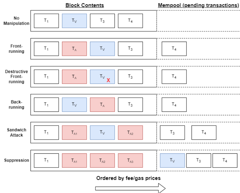
Fig. 60. Front-running and Miner Extractable Value. Attacker transactions are denoted T_A and marked in red, while the victim transaction is denoted T_V and is marked in blue. When destructive front-running occurs, the victim's transaction becomes invalid and fails to execute.
