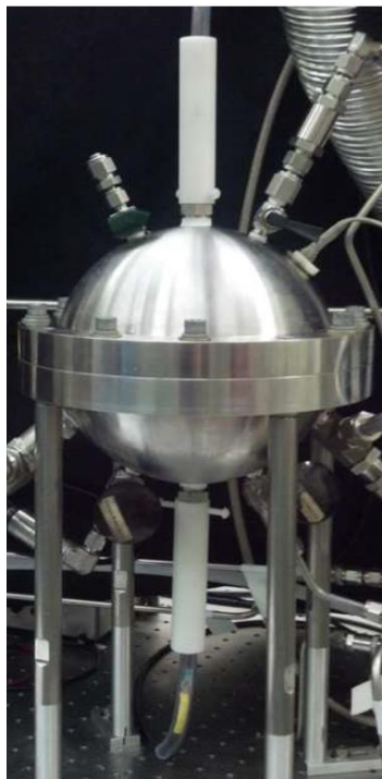
Figure A.2-1. Spherical 2-L chamber for JHPGL tests and constant volume method laminar burning velocity measurements
