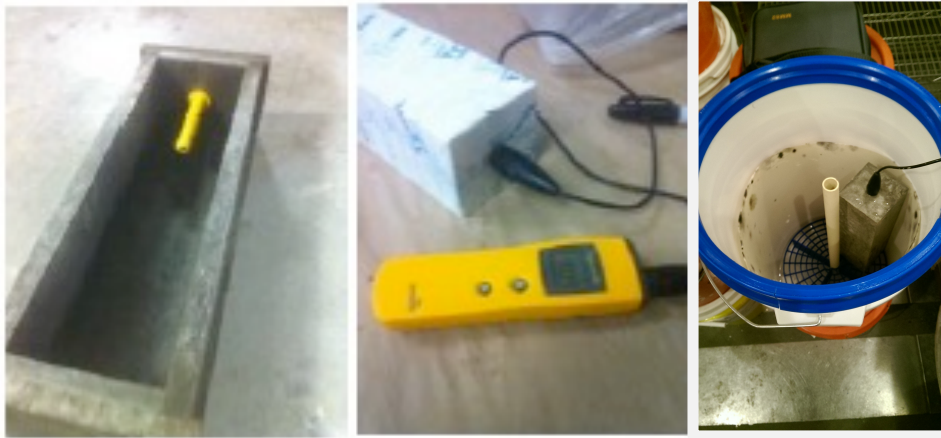
Figure 4-12. Details of (left) the RH probe insertion tube to be cast in a prism, (middle) the RH measurement apparatus attached to a sealed specimen, and (right) the measurement arrangement for prisms stored in lidded pails.
