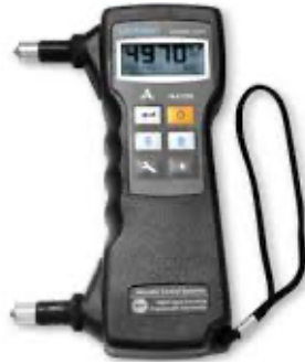
Figure 4-29. Image of UK1401 ultrasonic tester used to measure pulse velocity in prisms and cores.
