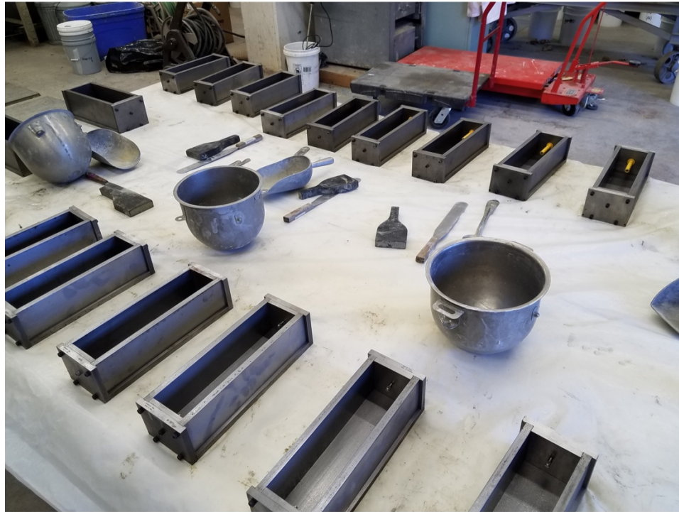
Figure 3-1. Layout of prism molds and tools in preparation for the Task 1 casting.
