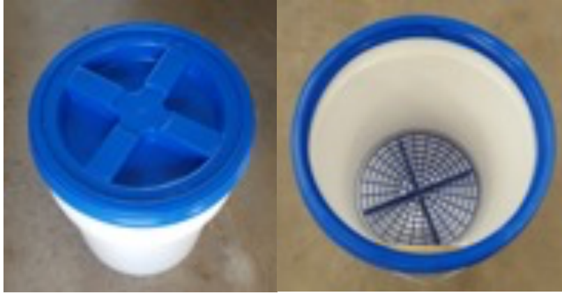
Figure 4-2. The sealed buckets modified for improved ASR expansion measurements have concrete prisms suspended over 1.8 L of deionized water and are lined with wicking blotter paper to provide a >95 % RH environment along the entire length of the prism columns.
