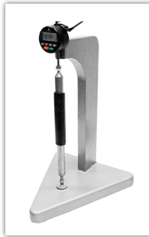
Figure 3-3. Setup for measuring prism expansion, with Invar reference bar
