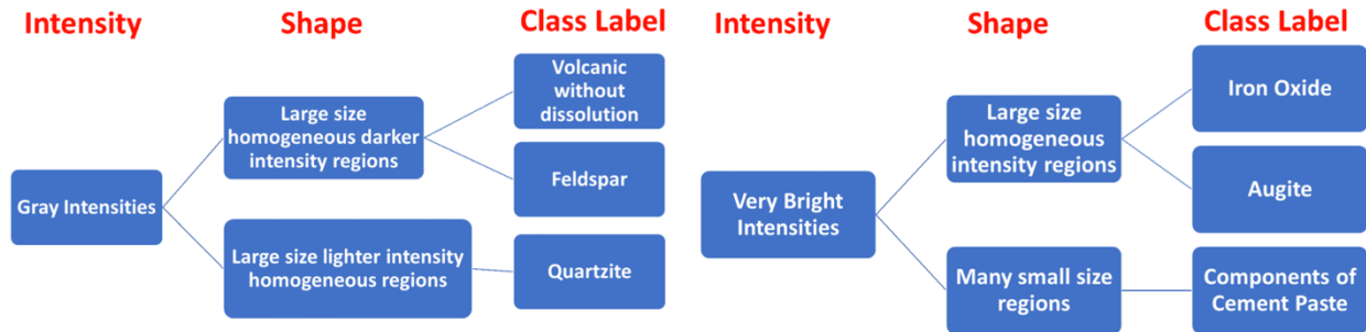
Figure 5-16. Visual description of contextual sub-classes based on SEM intensity and shape characteristics for gray (left) and very bright (right) image intensities and shape characteristics.
