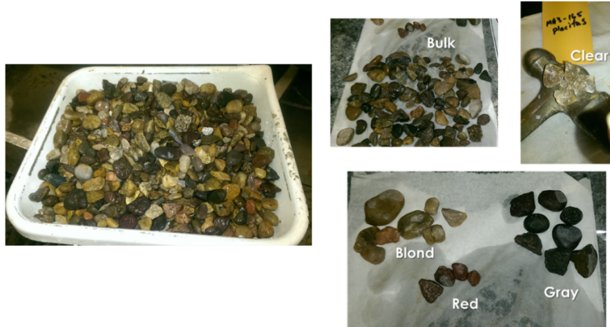
Figure 2-2. Placitas coarse aggregate components. Blond, red, and gray aggregate are volcanic components; clear are orthoquartzites.
