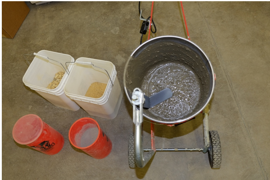
Figure 2-9. Pail mixer used to develop concrete mixtures.
