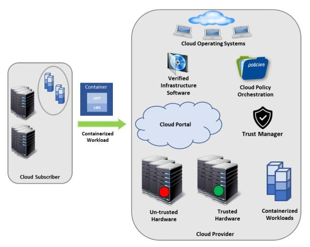
**Figure 1: Concept of Trusted Compute Pools**
