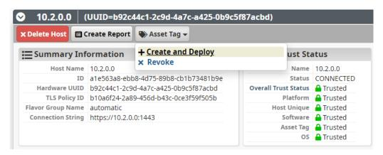
Figure 14: Example of Creating and Deploying an Asset Tag
