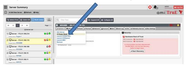
Figure 16: Example of Remote Power Control
