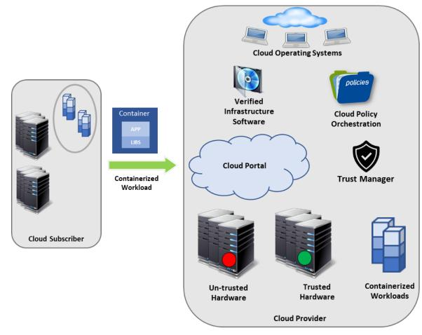
Figure 1: Concept of Trusted Compute Pools
