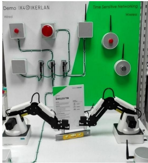
Figure 2. Wireless TSN applied to collaborative robotics
