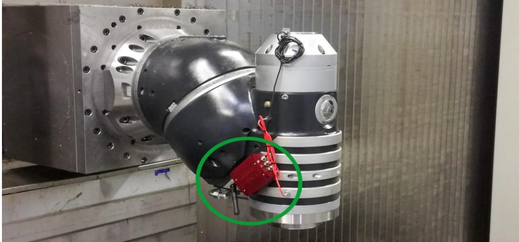
Figure 1. Milling machine monitored by a wireless sensor (Courtesy of SORALUCE-IDEKO **).
