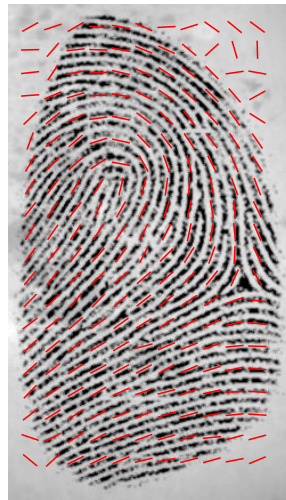
Figure 15. Synthetic fingerprint showing vector field of estimated ridge orientations.
