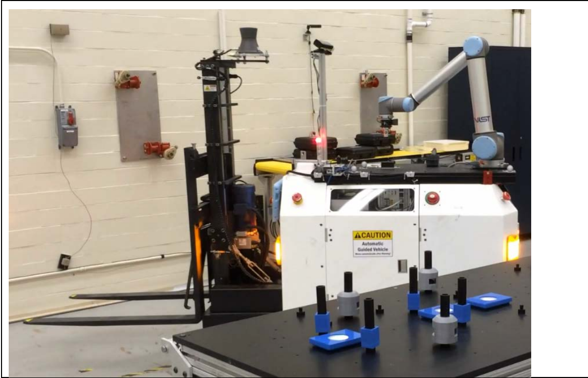
Figure 1: NIST AGV with onboard manipulator (background) moving to dock with a NIST reconfigurable mobile manipulator artifact (foreground).
