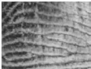
Figure 14 Demonstration of contrast reversal of contactless scanner
