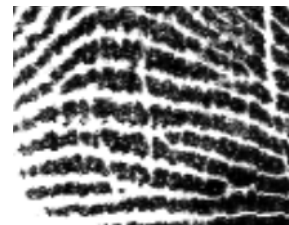
Figure 14 Demonstration of contrast reversal of contactless scanner
