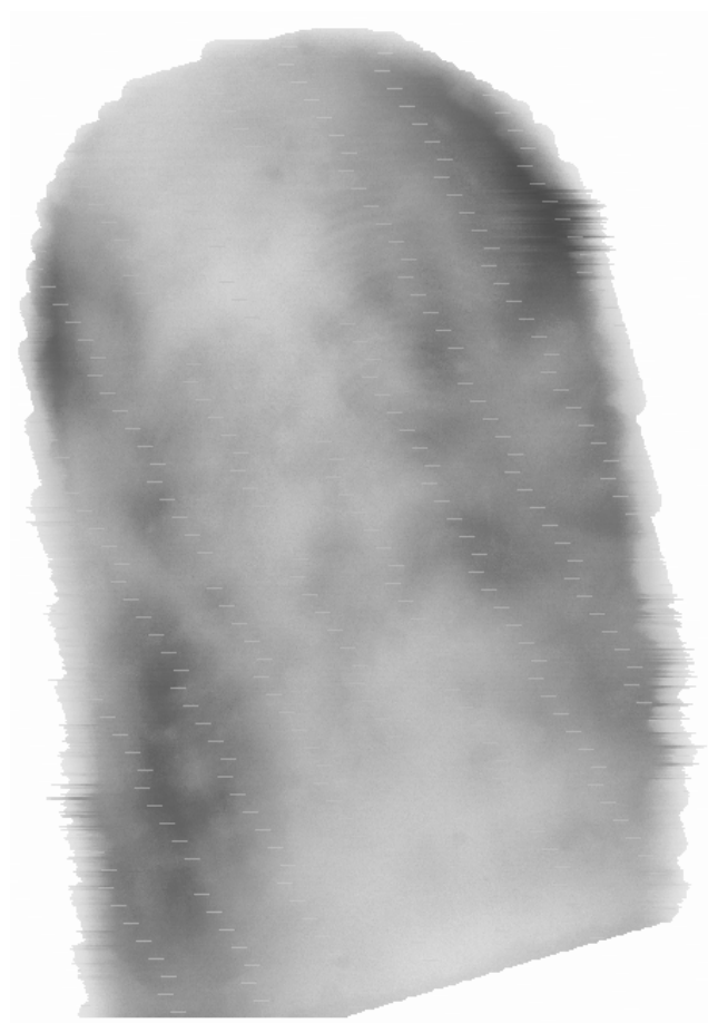
Figure 17 Example of complete loss of ridge detail observed with an image acquired with Contactless Scanner illustrating low BSNR value of approximately 15.
