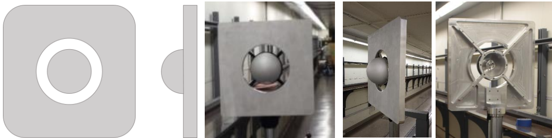
Fig. 2 Different views of the plate-sphere artifact used during the runoff
