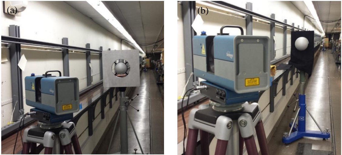
Fig. 12 Relative range tests showing a 3D imaging system placed in front of a) the plate-sphere artifact and b) the bare-sphere artifact. The laser tracker is at the far end of the tape-tunnel.
