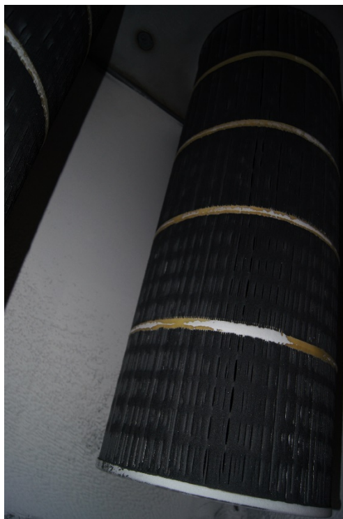
Figure 2. Soot covered the cartridge filters, looking upwards within the filter assembly box (see Figure 1). Some amount of light-color diatomaceous earth can be seen on the assembly wall surfaces behind and to the left of the filter.
