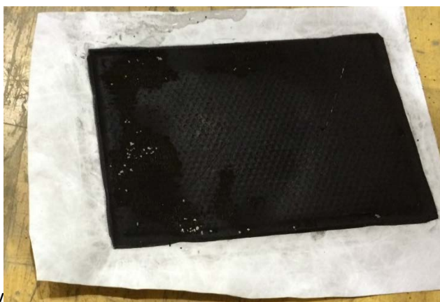
Figure 8. Soot “cake” on TYVEC filter media extracted from water using the pressurized filter apparatus shown in Figure 7.
