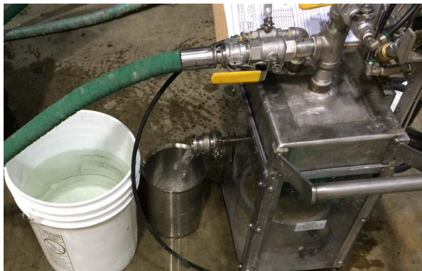
Figure 7. Pressurized filter device used to remove soot from the water. Filtered water (soot removed) is seen in the bucket and flowing from the device.
