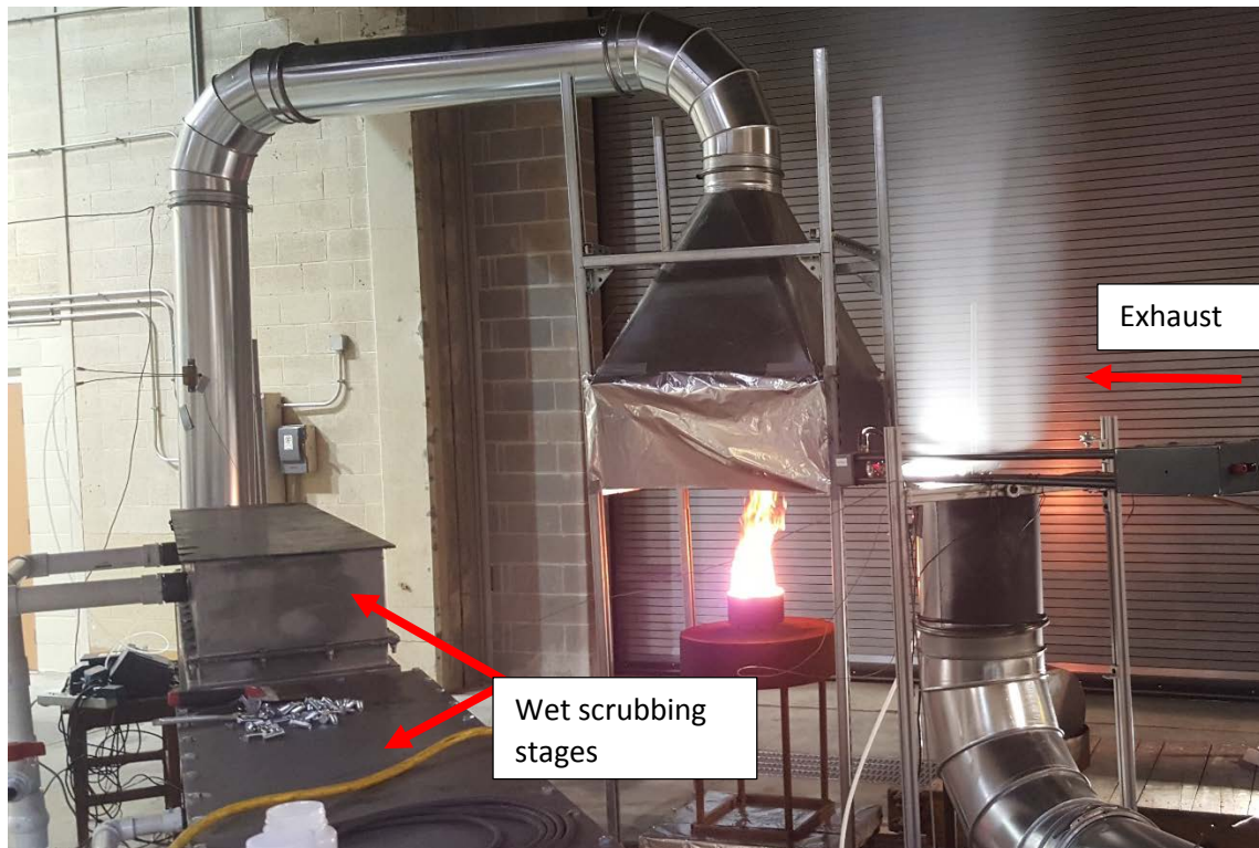
Figure 3. Toluene pool fire burning during the second soot filtering experimental series conducted in the NFRL on November 24, 2015. A visible smoke plume was observed at the illuminated vertical exhaust duct as seen on the right side of the image.
