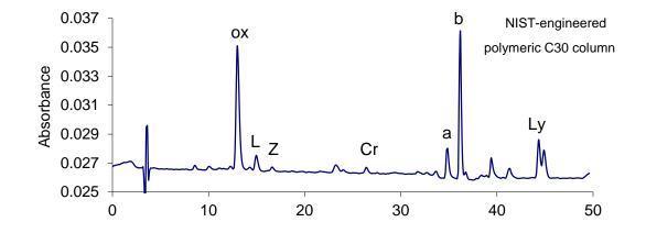
ox = trans- $\beta$ -apo-8'-carotenal oxime (internal standard) L = lutein Z = zeaxanthin Cr =  $\beta$ -cryptoxanthin a =  $\alpha$ -carotene b =  $\beta$ -carotene
