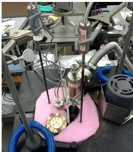
Figure 2. The setup showing the test chamber immersed in the water comparison bath with the SPRTs.
