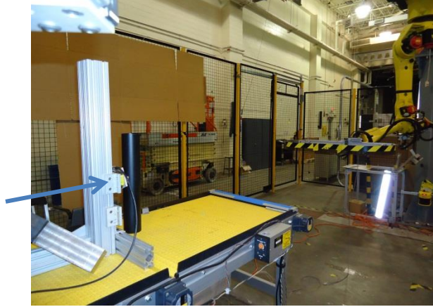
Figure 5: Single load cell, marked by an arrow, used with the initial test apparatus and robot.
