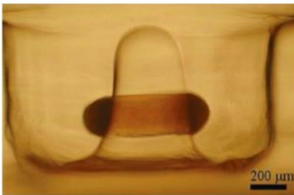
Figure 20. Side view of a toroidal cell cluster climbing the side of a conical pillar.
