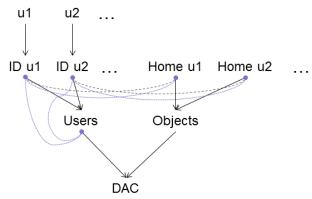
Figure 10: Authorization Graph for the DAC Operating System
