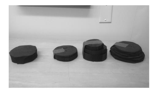
Figure 6: Prototype foam stacks cut with scissors. Final cut stacks would use cutting dies for uniform shape and size.
