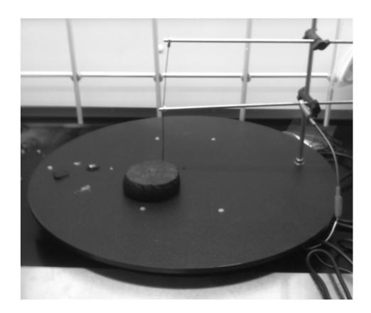
Figure 5: Hot wire foam cutter used to cut foam.
