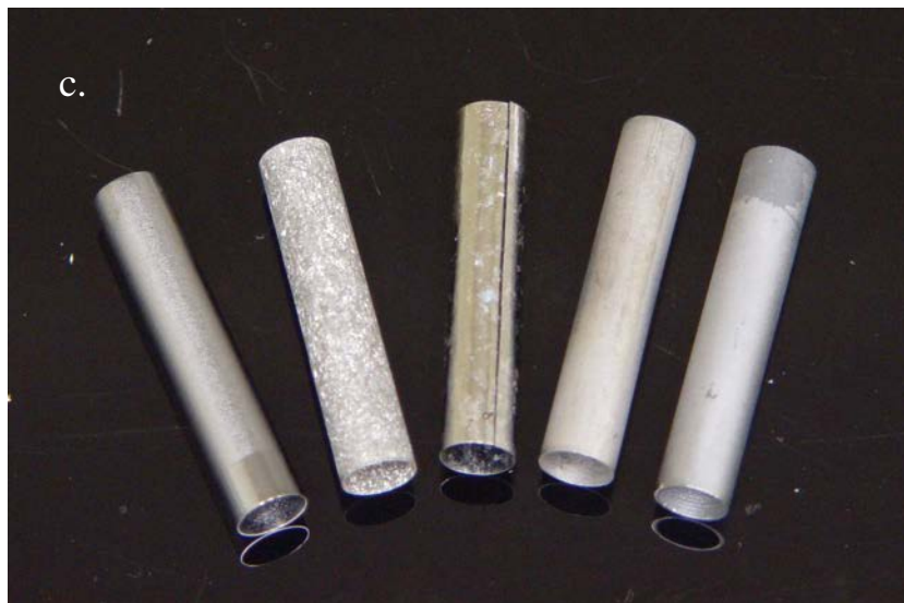
c. Different materials and methods of forming cathodes have been explored by Wink et al. (1993) and NIST. Examples of these cathodes are shown in the photo. The cathodes at each end are made of silicon and were provided by Max Plank Institute. The second from the left is a Fe-sintered cathode. The center cathode is made of Fe foil treated and rolled as described in the text and photos above. The cathode to its immediate right was cut from solid HP Fe rod using electrical discharge machining (EDM).
