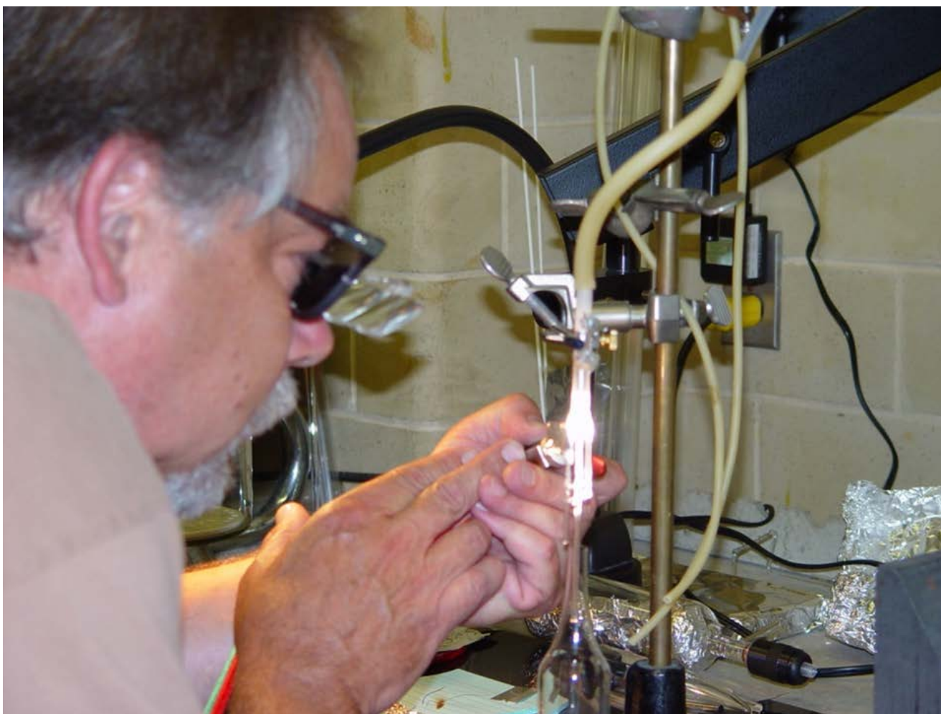
Figure 38 Quartz to W (anode) wire seal. The procedure for collapsing the quartz tubing around the W anode wire is identical to the procedure for sealing the cathode wire in place. After the seal, electrical continuity is tested between the Ni/Cr wire spring – positioned in the rear plug – and the anode wire exiting the quartz seal.
