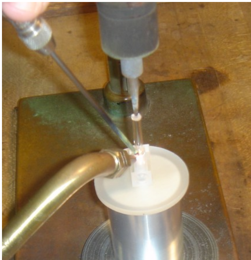
Figure 12 Optical fusing of tubes to a stopcock barrel. Tubes are optically fused to the barrel ports at a much lower temperature than typically used to fuse quartz to minimize distortion. Photo shows a quartz tube aligned with a bore hole on the barrel and held in place. A natural gas flame is uniformly applied to the transition between the tube and barrel.
