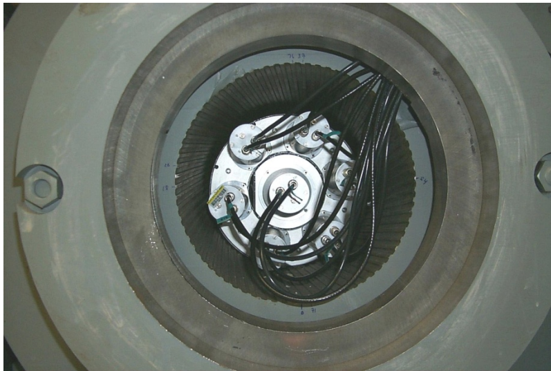
Figure 55 NIST llc system: active and passive shielding. NaI(Tl) coincidence (guard) detector specifications are comparable to HPGe \gamma -ray detection systems for anti-Compton suppression for high sensitivity (Heusser G, 1991). Passive shielding is a World War I gun barrel.
