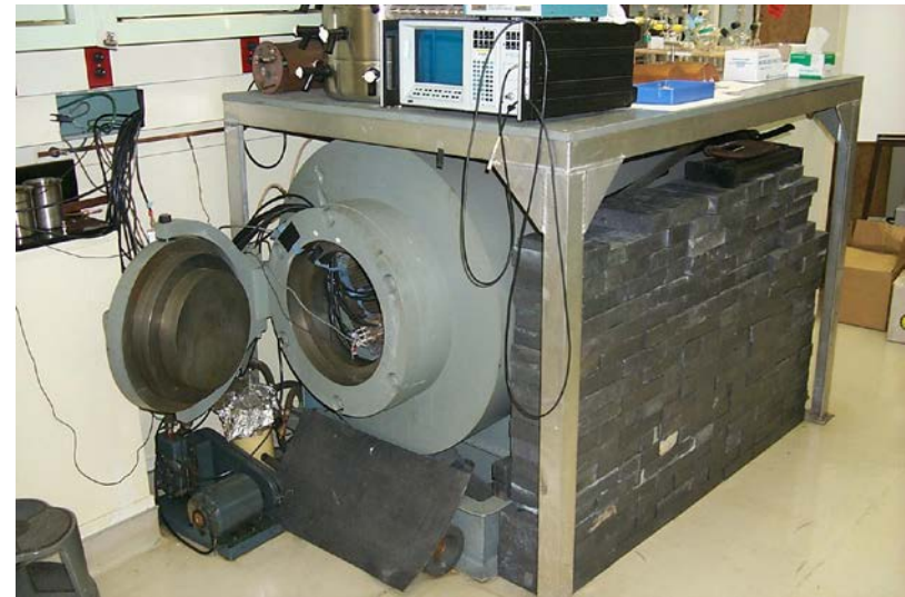
Figure 55 NIST llc system: active and passive shielding. NaI(Tl) coincidence (guard) detector specifications are comparable to HPGe \gamma -ray detection systems for anti-Compton suppression for high sensitivity (Heusser G, 1991). Passive shielding is a World War I gun barrel.
