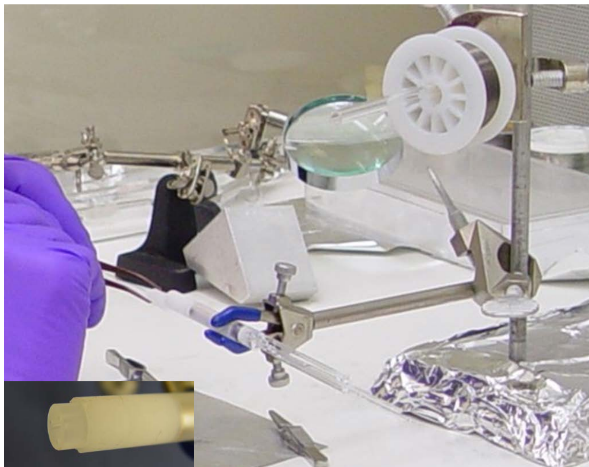
Figure 36 Securing the anode wire within the GPC body. Thread a 50 \mu\text{m} diameter W tether wire (25 cm long) through the center tube and out the body using the same technique to insert the cathode lead. The tether wire is now glued to the 13 \mu\text{m} diameter W anode wire. Allow at least an hour for the glue to set and outgas. Very slowly begin to pull the anode wire through the counter while moving the plug and spring toward the body with some tension on the anode. Inset at lower left shows the plug after it has been inserted into the body. Continue to push on the plug and maintain tension on the W wire.
