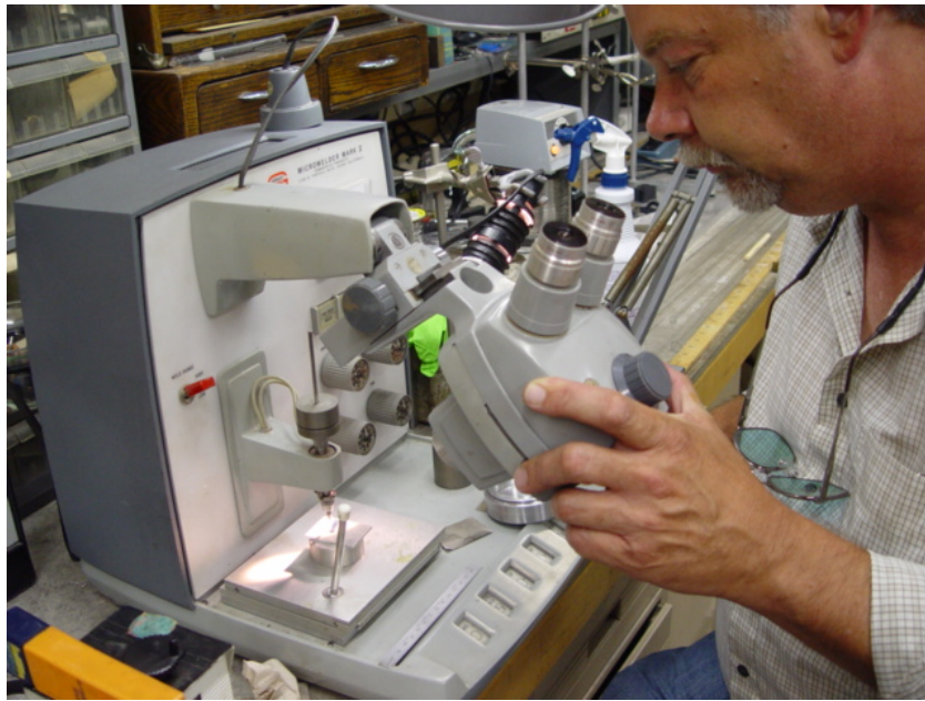
Figure 26 Spot welding a W-wire burr to a Fe cathode. A 50 \mu\text{m} diameter W wire is spot welded to the Fe foil cathode near its seam and at one end. The left photo shows the micro welder with microscope. The right image shows the W wire spot welded to the Fe foil before it is brightened by annealing.
