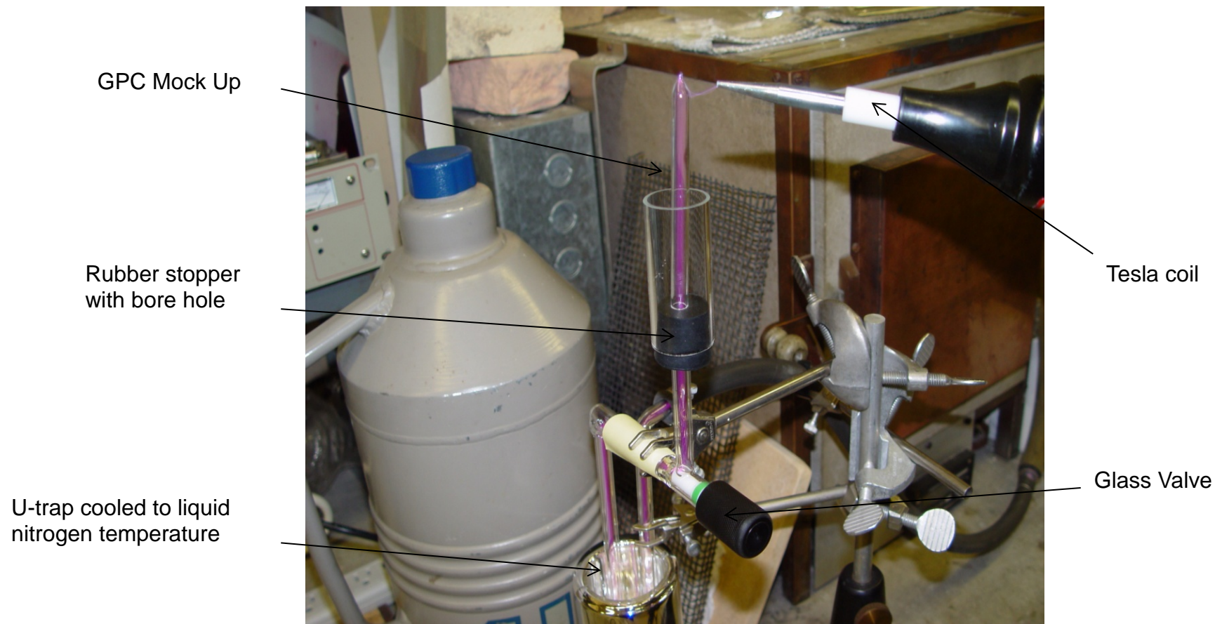
Figure 22 Leak testing the GPC envelope. A vacuum system and Tesla coil apparatus is used to leak test the seals that connect the body, front plug and tubes together in preparation for counter assembly. The photo shows a cold trap, a glass valve and rubber stopper used to establish a vacuum in the GPC envelope; here simulated by the vertical tube above the stopcock. The GPC is inserted through a hole bored in the center of the rubber stopper. While drawing a rough vacuum (1 Pa) on the GPC, a Tesla coil is positioned near a seal. If a hole exists in the quartz, then the arc discharge will be directed through it from the tip of the Tesla coil (purple arc).
