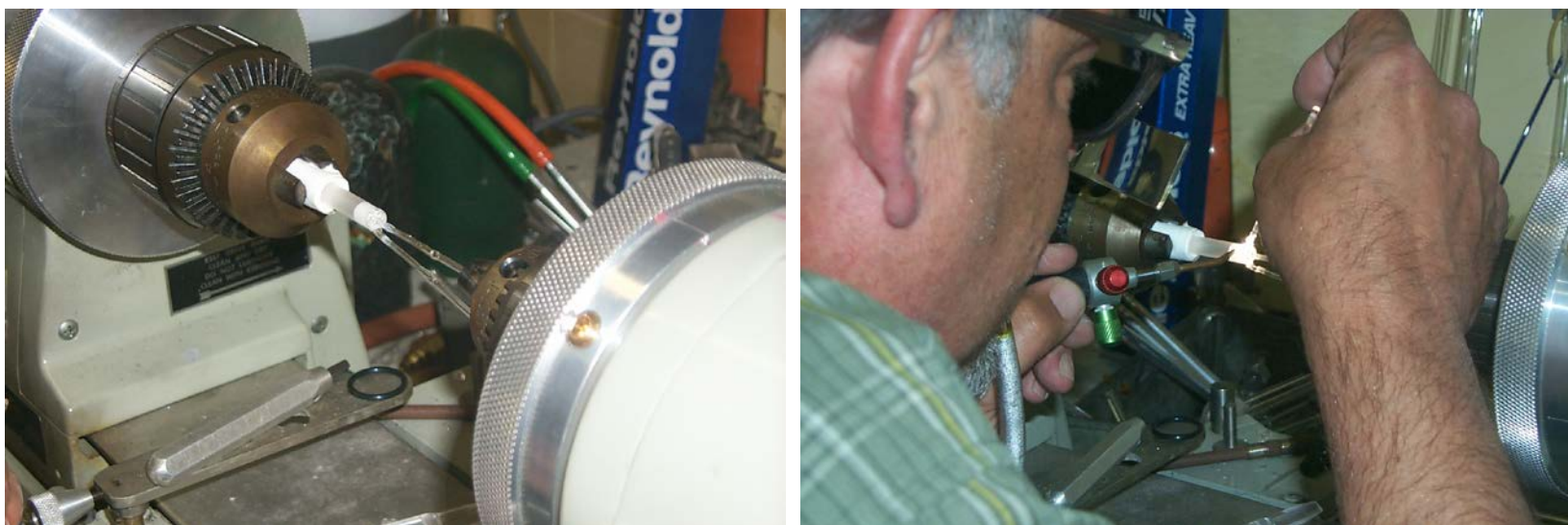
Figure 20 Sealing the outside capillary tubes to the GPC body. The passage way is blown open to accommodate the high voltage lead. A capillary tube of the same dimension as the center tube is sealed at a small angle and in line with this outside channel of the plug (left). The other passage way is blown open to accommodate the gas inlet. A third capillary (same diameter) is sealed to the front plug over the remaining channel for the gas inlet via the stopcock.
