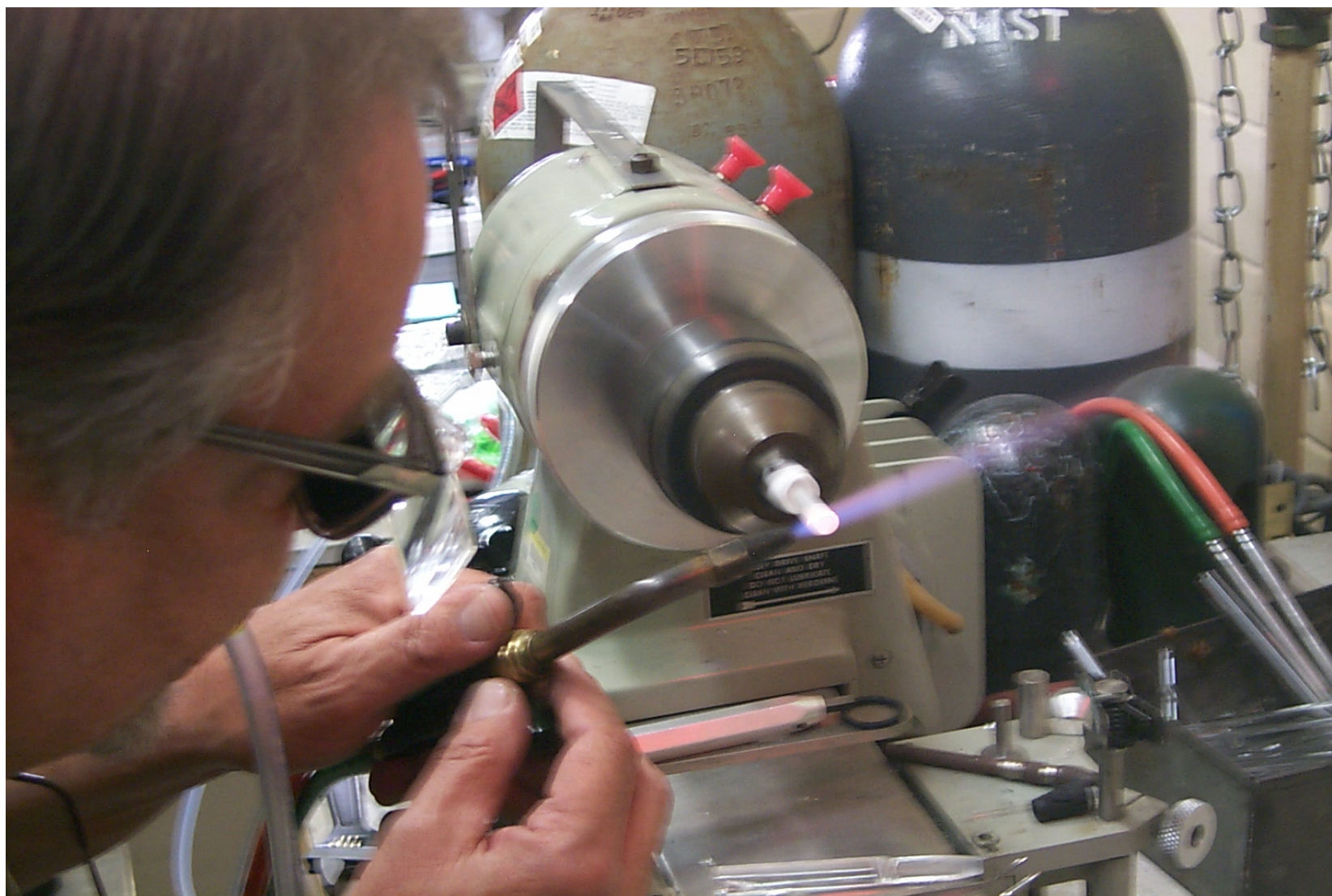
Figure 18 Sealing the front plug to the GPC body. The glass blower is shown sealing the front plug to the edge of the GPC body using a H_2/O_2 flame.
