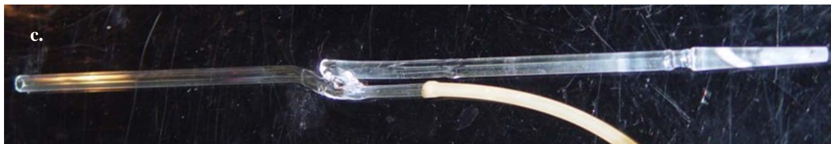
Figure 52 Jigs and tools. a. At the top left is shown counter bodies used to check the cathode dimensions, glass rods to roll Fe foil into cylinders for cathodes, glass tubes to support cathode while inserting into counter body, and tubing to guide tether wire through the high voltage capillary. b. Assorted tools are shown: e.g. , clamp tweezers, pencil vice, normal tweezers, scissors, needle-point probe and drill (in vial). c. The bottom photo is a jig used to align the stopcock barrel (right side taper) to the center point of the GPC (left side to be chucked in lathe).
