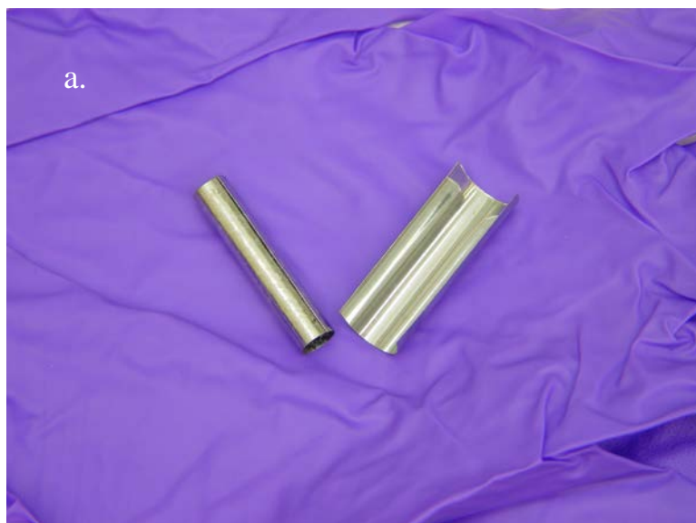
Figure 23 Fabricating cathodes. An Fe-foil cathode is shown here at three stages of shaping: a. initial rolled foil (right) with cylinder formed after annealing (left); b. rolled cathode friction tight within a tube to simulate a GPC; and,
