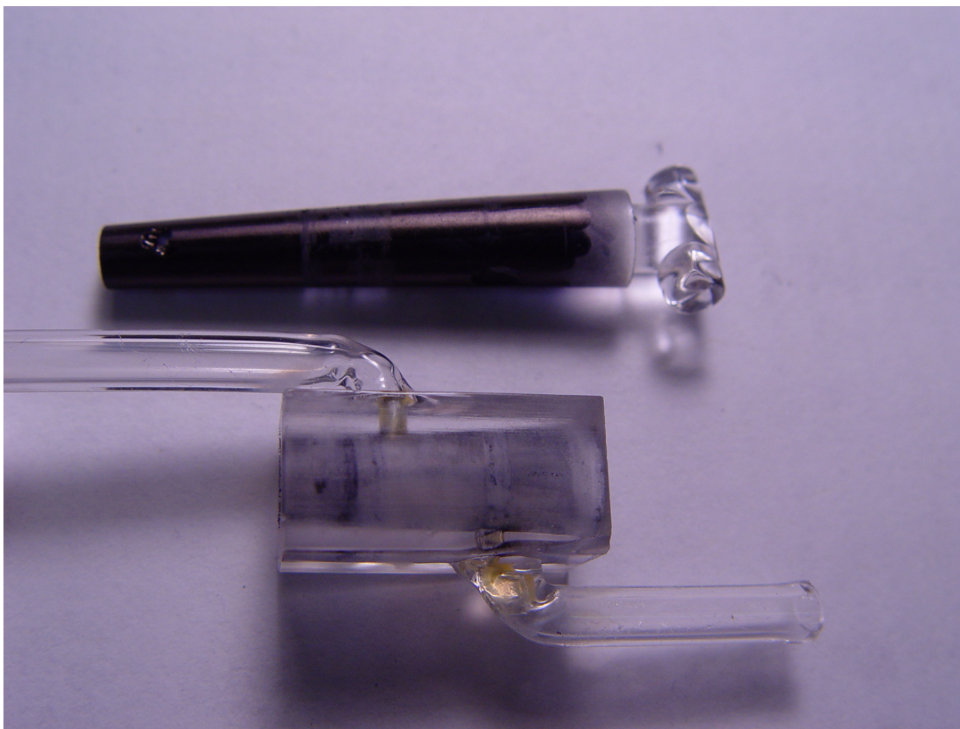
Figure 14 Inspecting stopcock lapped surfaces. Now the tubes are bent and the plug has a handle. The plug and barrel are tested by applying graphite to their surfaces and rotating the surfaces while in contact with each other. Any striations that appear suggest a potential path for gas leakage.
