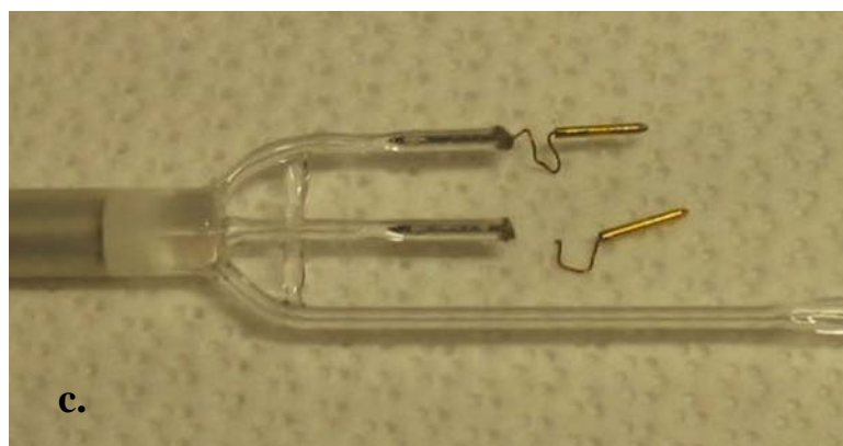
Figure 47 Examples of broken GPCs. a. catastrophic breakage from an overpressure on the vacuum line; cannot be repaired but the plugs can be salvaged. b. inlet tube to the stopcock was broken by applying too much torque to the stopcock plug when turning without sufficient support of the barrel – difficult to reseal tube to the barrel without distorting the taper. c. an electrode connection is broken most likely due to metal fatigue – relatively easy to fix by boring a hole through the epoxy and Ga then securing a new connector wire in the Ga using conductive silver epoxy. d. an anode wire is broken from extensive vibrations as the GPC was mounted via an o-ring fitting on a glass vacuum manifold connected to a He-cryopump system.
