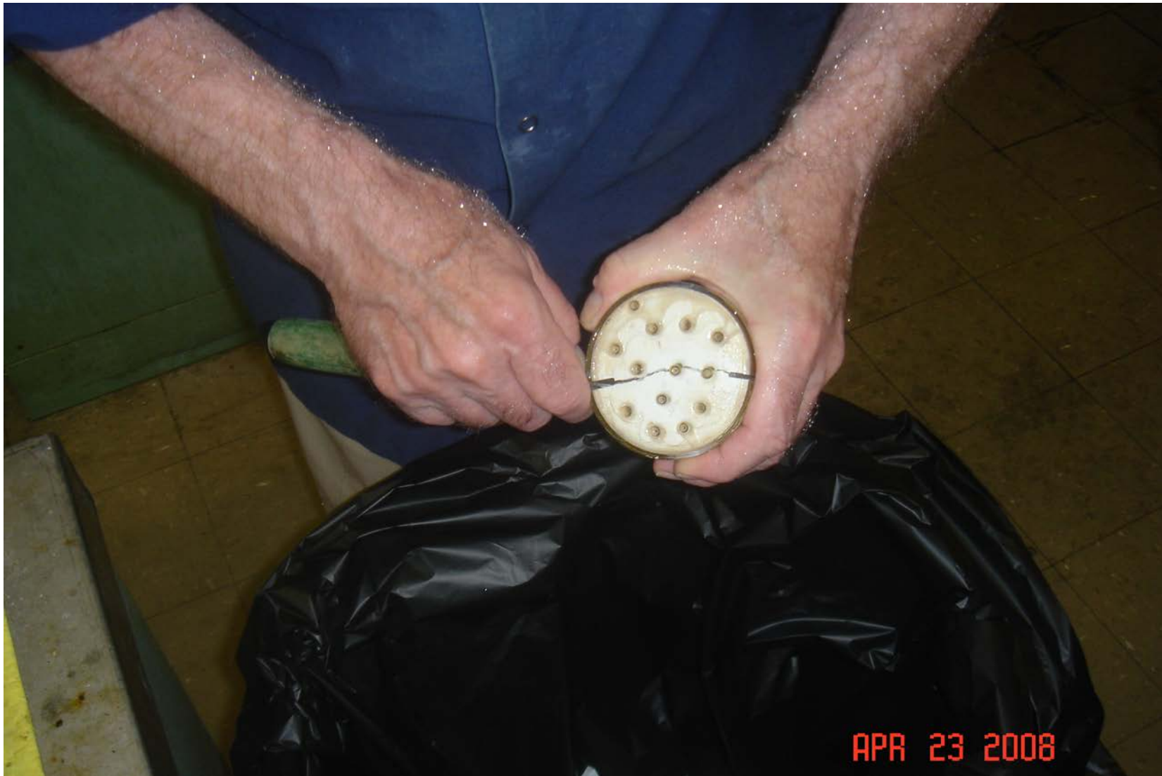
Figure 10 Stopcock tubes mounted for grinding and polishing. Several quartz tubes are held in a glass ring using gauging plaster. Tube ends are ground and polished to an optical finish for later fusing to stopcock barrels. The photo shows the tubes being demounted.
