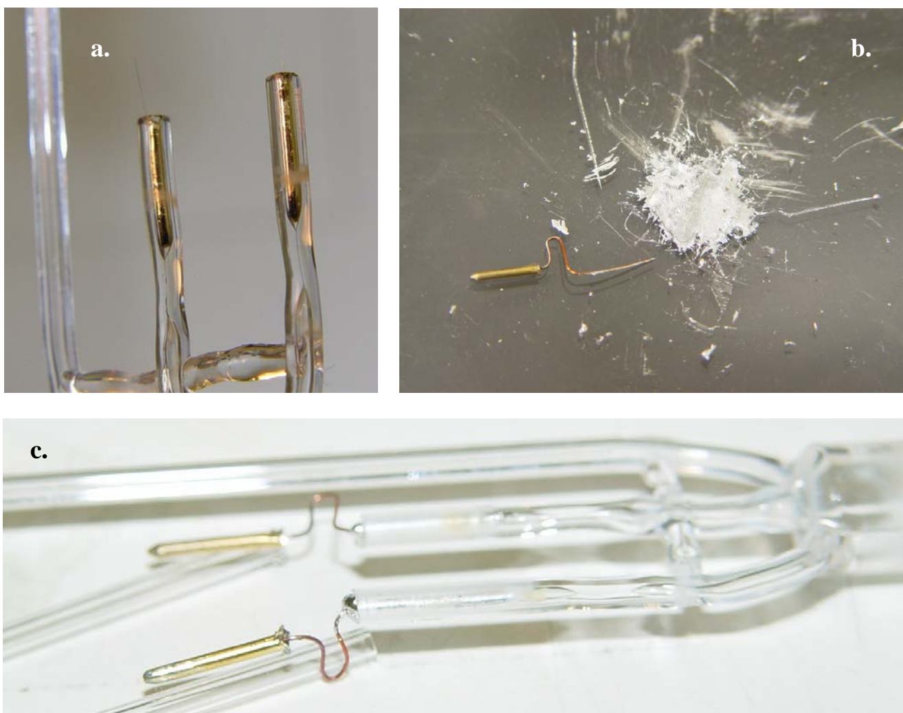
Figure 50 Gallium welded electrical connectors. a. Photo shows the quartz to W-wire seals made of the anode wire (center tube) and the cathode-lead wire (right tube). Each tube end is filled with Ga using a pipette (Figure 49). b. Copper leads should be wetted with Ga before inserting in the tube well filled with Ga. c. Copper leads are then slowly pushed into each well. If a cradle is available, the counter can be fit to it to test if the leads are of suitable shape and length.
