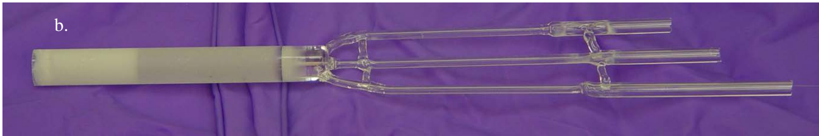
Figure 16 GPC configuration for vacuum leak testing seals. a. GPC dimensions (top) are shown for the counter to conform to the cradle cavity. The top tube (#3) shows a bubble for the seal to connect the stopcock. The three tubes terminate with 3.2 mm outer diameter tubing to connect to an o-ring fitting for vacuum leak testing of each quartz-to-W seal. Tubes are tested in the order stated. b. The photo is of an assembled body, front plug, and tubes. Note that the body has been sealed against the plug to minimize virtual leaks. Side channels for the gas inlet and HV have been blown out to the side at the edge of the body. Especially important is a gradual transition from the HV channel to the capillary tube. This facilitates the threading of a 50 \mu\text{m} diameter tether wire through the HV channel and tube that will be used to pull the cathode W-wire lead through the assembly.
