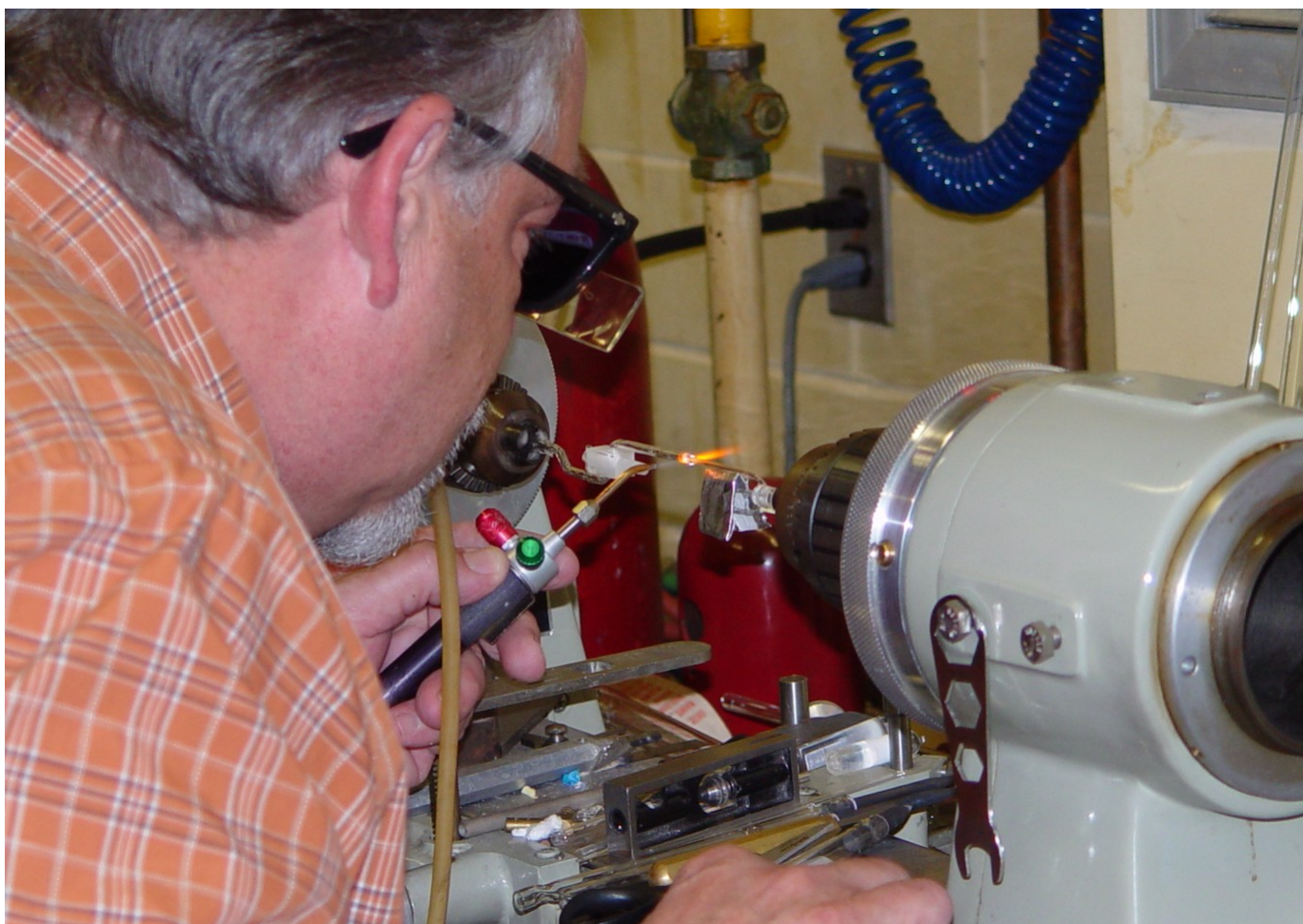
Figure 43 Sealing a stopcock to a GPC - step II. The counter and stopcock are fused using a H 2 /O 2 flame. Electrodes or W-wire leads are shielded from the flame with Al-foil-covered high temperature ceramic fiber (left of flame). The counter tube is preheated slightly before fusing the tubes in an attempt to drive most of the moisture left to the stopcock side. The purpose is to minimize the amount of moisture that will migrate to the virtual leaks within the GPC.
