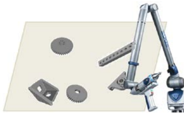
Figure 14. 3D coordinate measuring system for parts localization.
