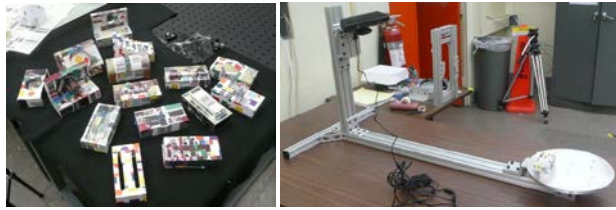
Figure 13. The artifacts used in the challenge and the ground truth rig with the sensor mounted at top left. [Permission granted by the author [11] to use the Figure]
