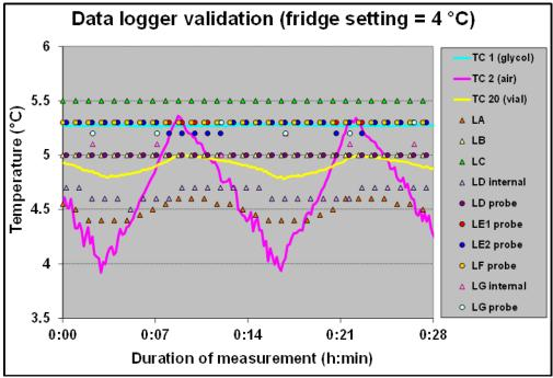
Fig. 3. Selection of temperature data from a thermocouple comparison test with refrigerator set to  $4 \,^{\circ}$ C.
