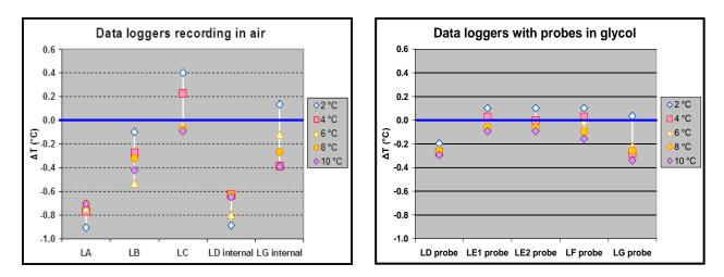
Fig. 4a, 4b. Data logger temperature offset from reference thermocouple at different refrigerator temperature settings (2 °C, 4 °C, 6 °C, 8 °C, 10 °C).
