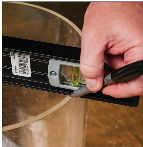
Figure 3-28. Marking Evenly Spaced Measuring Points Across the Top of the Test Measure
