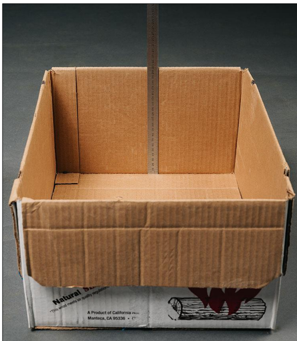
Figure 3-8. Measuring the Internal Height of the Box
