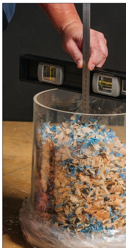
Figure 3-29. Placing the Ruler into the Test Measure with Zero End Down
