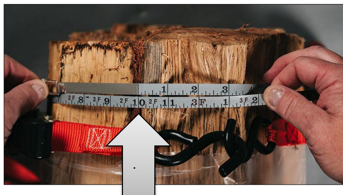
Figure 3-16b. Measuring the Circumference of the Bundle At the point of the arrow, the circumference of the bundle is 2 ft 10 in (34 in).
