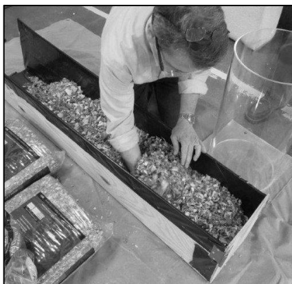
Figure 3-20. First Pour into the Test Measure.
