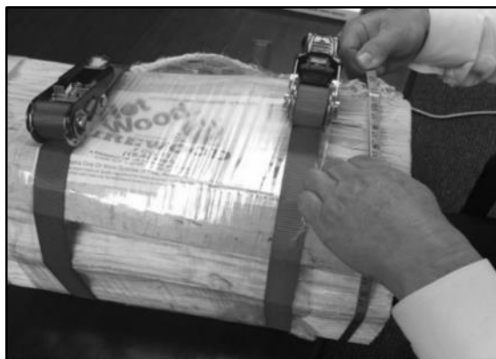
Figure 3-13a. Strapping the Ends of a Bundle.
