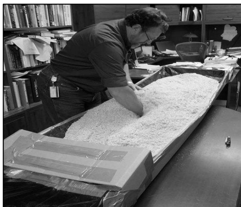
Figure 3-18. Spreading Bedding Material
